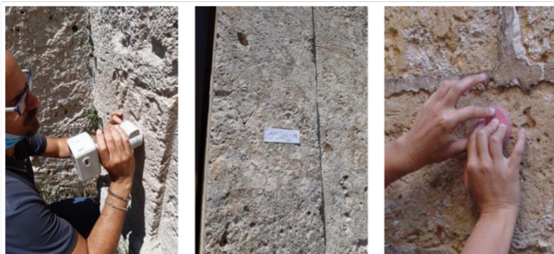
Figure 15. Non-invasive and cost-effective diagnostics to evaluate products behaviour. Colorimetric Test on the left; Scotch Tape Test in the middle; Water Absorption on the right.
