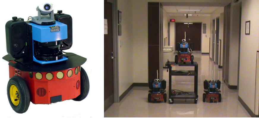
Figure 3.20: The experimental setup at Distributed Intelligence Laboratory of University of Tennessee. On the left: a zoom of a Pioneer-2Dx mobile robot. On the right: the whole setup.
