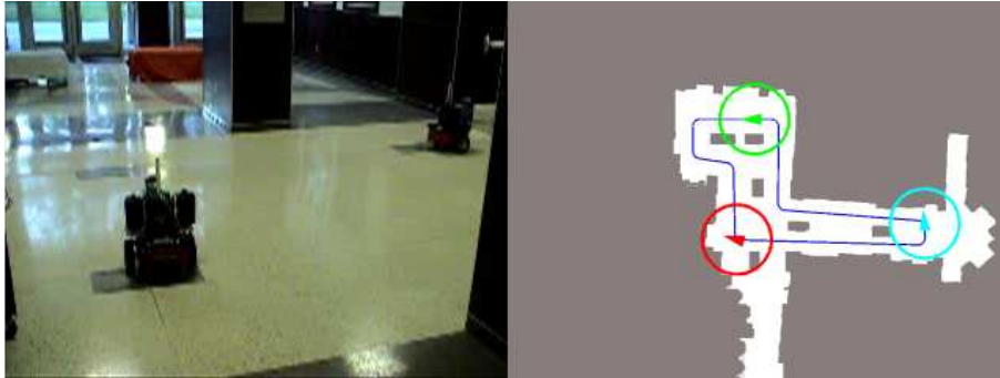
Figure 3.25: On the left a portion of the environment. On the right its representation obtained by Player/Stage software, the path and the three patrolling robots.
