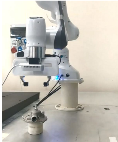
Figure 3.12: Robot and camera setup for data acquisition.
