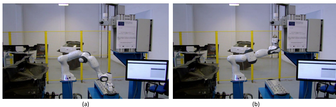
Figure 2.35: Big Head picking form the kit (a) and application of glue by using the dispenser (b).
