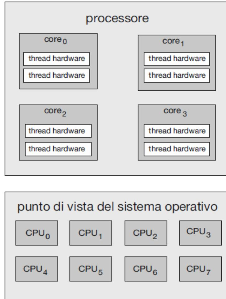
Figura 5.14 Chip multithreading.
