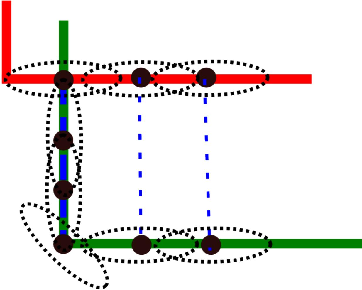
All of the points along the vertical section of the green scan are incorrectly associated with a single point in the red scan
